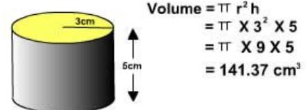
$$\begin{aligned} \text{Volume} &= \pi r^2 h \\ &= \pi \times 3^2 \times 5 \\ &= \pi \times 9 \times 5 \\ &= 141.37 \text{ cm}^3 \end{aligned}$$
